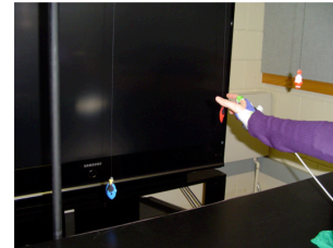
Figure 2: “Dangling Fish” used to measure speed of reach. The position tracker is attached to the subject’s hand.
