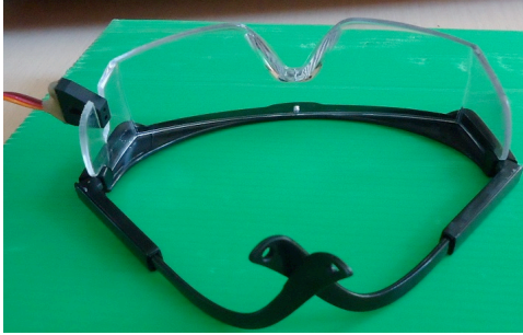
Figure 5 - Glasses adapted to the optical sensor, showed at the left side of the photo
