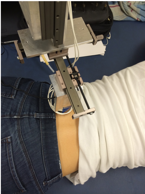
Figure 10. Indentation test on lower back.
