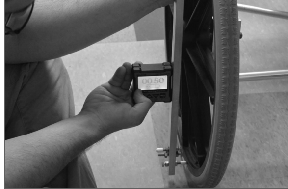
Figure 2 – Misalignment and Inclinometer Measuring Camber Angle
