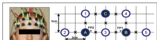
Figure 1: Source-detector configuration. Each solid circle represents a detector, while each open circle represents a source-pair consisting of one 690 nm and one 830 nm source fiber.
