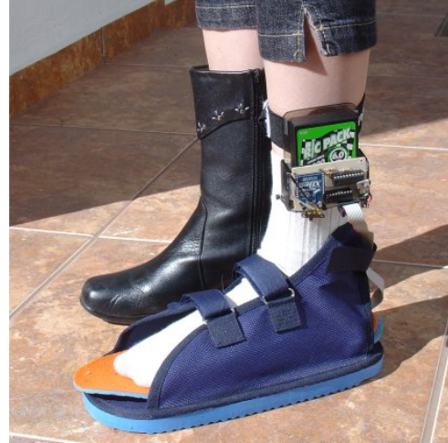
Figure 2: Fully wearable device with on-board battery and RF receiver.
