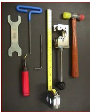
Figure 7: Simple tools are all that is necessary to build CREFORM devices.
