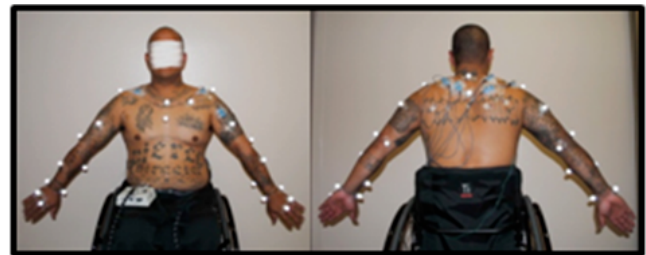
Figure 3: Reflective markers for tracking the upper extremities segment kinematics.
