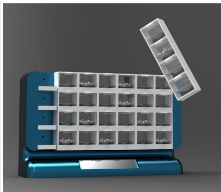
Figure 2: A 3-D image of The Smart Pill Box with a column removed.
