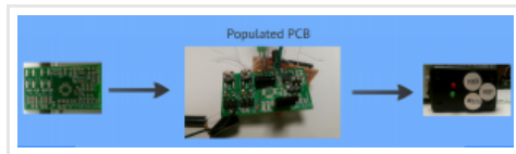
Figure 6: Printed PCB (left), populated PCB, and after packaging
