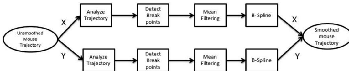
Fig. 2. Overall smoothing process in APSS has four main steps. This technique process X and Y coordinate separately. Needed steps for smoothing for both X and Y coordinates are the same. First of all if user has any mouse movements then his trajectory will be analyzed to detect breakpoints coordinates. Later on in first phase of smoothing, the *Mean* filtering technique will reduce unsmooth points in trajectory. In the last phase B-spline technique will smooth and deliver final trajectory.
