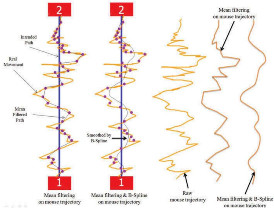
**Fig. 3.** Steps in smoothing mouse trajectory involve analysis of the mouse trajectory and break points detection. Then in the next step, the detected break point will be fed into the *Mean* filtering step to eliminate large noise disturbances from the trajectory. The final step recalculates the mean break points, which will then be passed to B-spline. Once all these steps are completed, a smoothed trajectory will be sent to the computer to be displayed on the computer screen.
