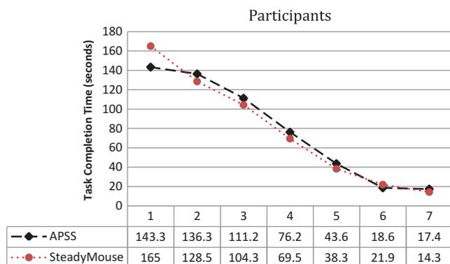
**Fig. 7.** The x-axis is the Task completion times (TCT) using adaptive path smoothing via B-spline (APSS) and SteadyMouse. Participants had different TCT in comparison to each other. However, comparison between the two techniques shows similar TCT for each participant.
