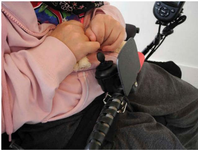
Figure 3. MEC joystick.
