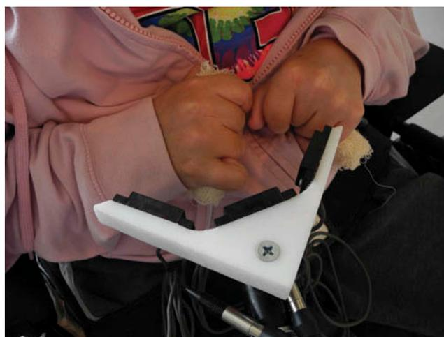
Figure 2. Custom proximity switch array.
