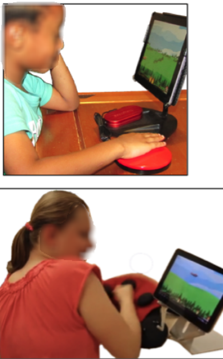
Figure 1. Top: TabAccess, Bluetooth switch interface for tablets, Bottom: Bluetooth plush switch used in sessions with children with disabilities
