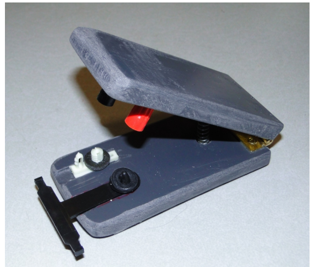
Figure 4. Stapler design for pressing the washer onto the post. The grooves in the base align the posts beneath the hollow cylinders in the top arm of the device.
