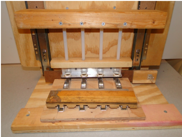
Figure 5. Press designed to simultaneously produce four dial assemblies.
