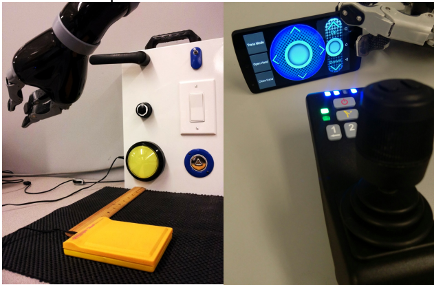
Figure 3: the Jaco ARM and ADL Task Board (left) and touch-joystick control interface and the original joystick controller (right)
