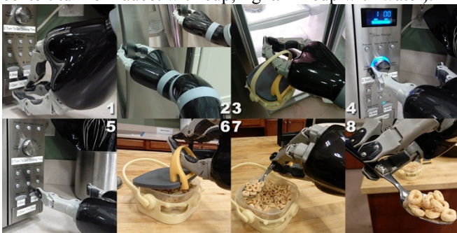
Figure 3. Preparing and then having a simple meal sequence (1: push microwave door open button, 2: open refrigerator door with jammed fingers in the upper right picture, 3: take out the container, 4: set timer to 1 minute using knob, 5: push start button, 6: open container cover, 7: scoop food, 8: bring food to mouth).
