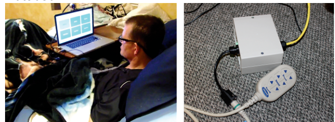
Figure 1. Henry Evans using the Autobed via a web-browser and his existing head-tracking HCI (left). The Autobed module and bed's control pendant (right).
