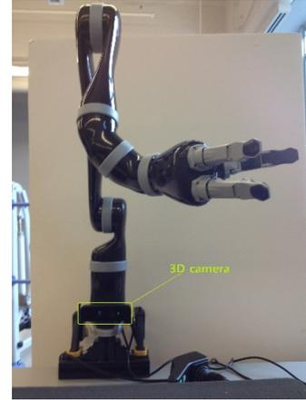
Figure 1. JACO with Senz3D camera
