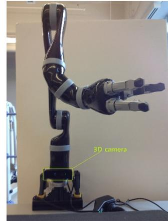
Figure 1. JACO with Senz3D camera
