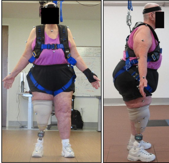
Figure 1: Vicon full body Plug-in-Gait model marker placement on the transtibial amputee wearing a K3 Catalyst foot.
