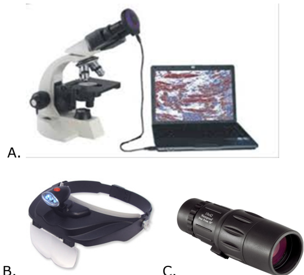
Figure 1: A. Digital video camera mounted on a light microscope connected to a computer monitor used for histology and cytology activities. B. Head loupe for gross anatomy, surgical procedures, dentistry, and other near observation tasks. C. Monocular for viewing gait behavior in horses and other distant activities.
