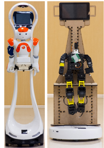
Figure 1: On the left, the system which we developed to explore the use of socially assistive robots in elder care facilities, it is a Nao robot on a VGo telepresence base. On the right, our work in progress for the lower cost Lil’Flo system.
