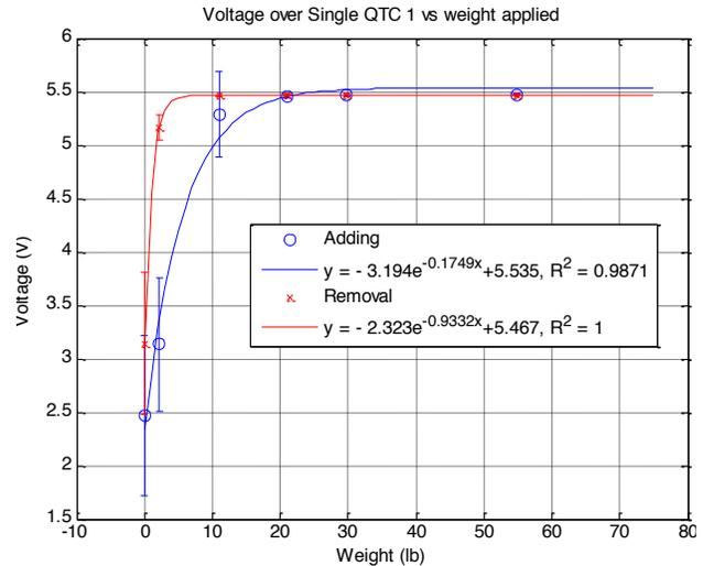
**Figure 4. Voltage vs weight of QTC Position 1 (Individual)**
