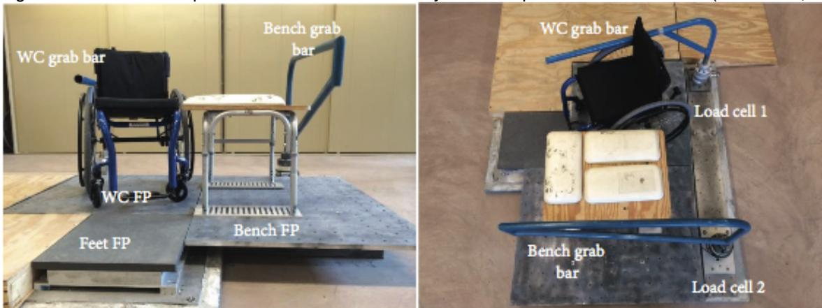
**Figure 1:** Front (a) and top (b) views of the transfer station. WC: wheelchair; FP: force plate.
