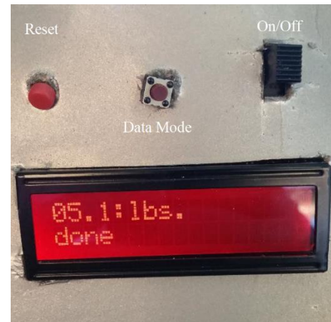
Figure 3 the control and display interface of ToeTronics Gen1.
