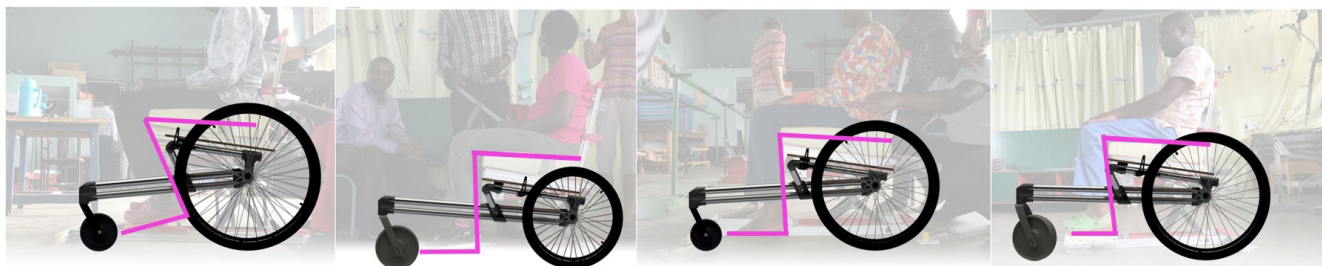
Figure 1 Wheelchair chassis of different configurations made according to the measurements and specifications collected from the clients.
