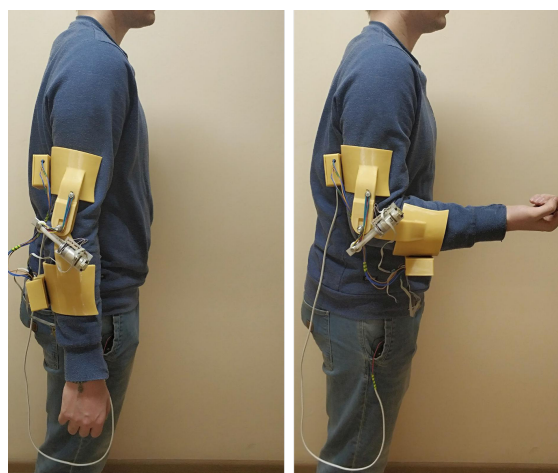
Figure 5 - Elbow orthotic with elastic elements and distance adaptation control system
