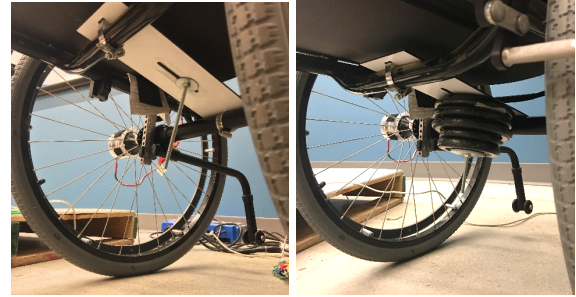
Figure 3. (Left) Dibond shelf to support weights at the center of mass. (Right) 4 kg added to the shelf.
