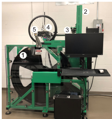
Figure 2: Drum-based rolling resistance testing machine. (1) Drum, (2) Upper Frame, (3) Arm, (4) Truck, (5) Load Cell
