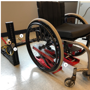
Figure 1: Laser measurement system for toe and slop. (1) Laser, (2) Constant Force Springs, (3) Lift Mechanism
