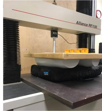
**Figure 1. Hysteresis test fixture**
