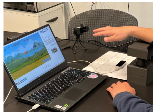
Figure 1: R3THA set up which includes: laptop, infrared motion capture camera, arm support, and video conferencing camera.
