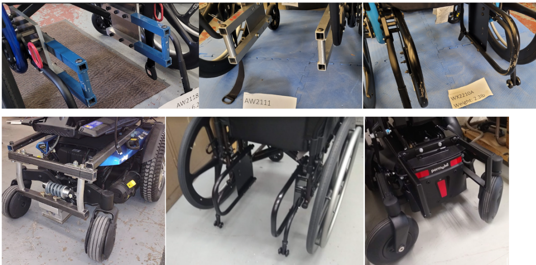
Figure 1. Photos of UDIG-compatible attachments for (from left to right, top row) Ki Mobility Catalyst 5 (versions K1, K2, K3), (bottom row), Quantum Rehab Q6 Edge 2.0, Sunrise Quickie 2, Permobil F3 Corpus.
