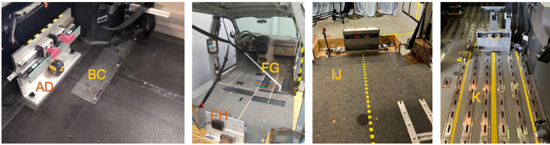
Figure 1. Setup for each wheelchair station. AD and BC were in a modified Dodge Caravan. For AD conditions, the anchor was located rearward and inboard of the wheel well, while BC (shown by mounting plate) placed the anchor more outboard and forward of the wheel well. Conditions E, H, I, and J simulated a second-row center position, while K was in a third-row outboard position. Conditions FG were in the front row right; the experimenter installed the UDIG anchor in place after they entered the vehicle.
