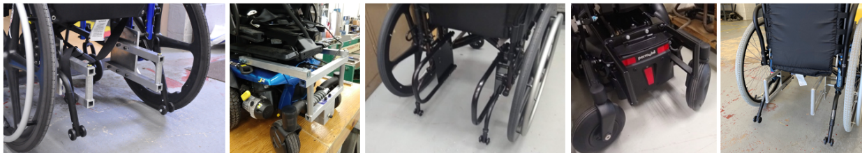
Figure 3. Photos of UDIG-compatible attachments for (from left to right) Ki Mobility Catalyst 5, Quantum Rehab Q6 Edge 2.0, Sunrise Quickie 2, Permobil F3 Corpus, and Motion Concepts Helios.
