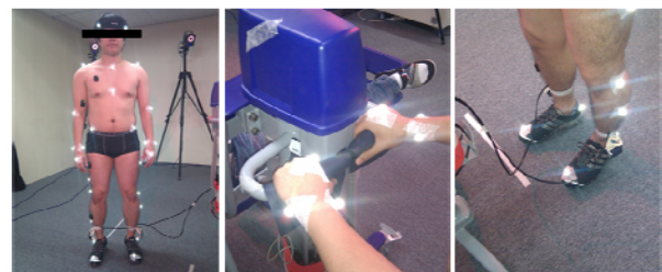
Figure 2: EMG analysis and pressure mapping system using 3D motion capture.
